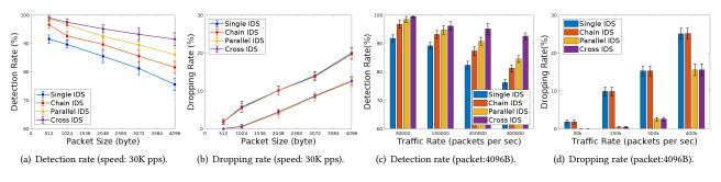
Figure 4: Evaluation of different configurations under varying speeds and packet sizes.
